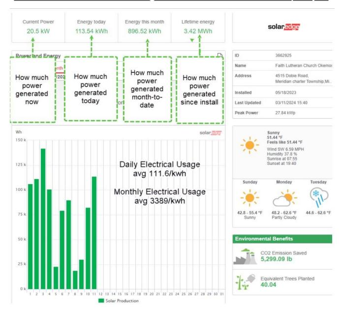
This shows every panel and the output kWh. It is monitored to verify all panels are working. If one drops below normal output then they will come out and replace it.
